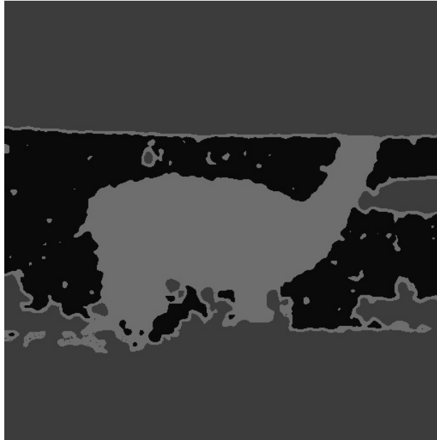
Figure 13: Result after clustering. The dark gray area represents the outside of mask. The darker area and the lighter area represent the 2 distinct regions inside the mask
